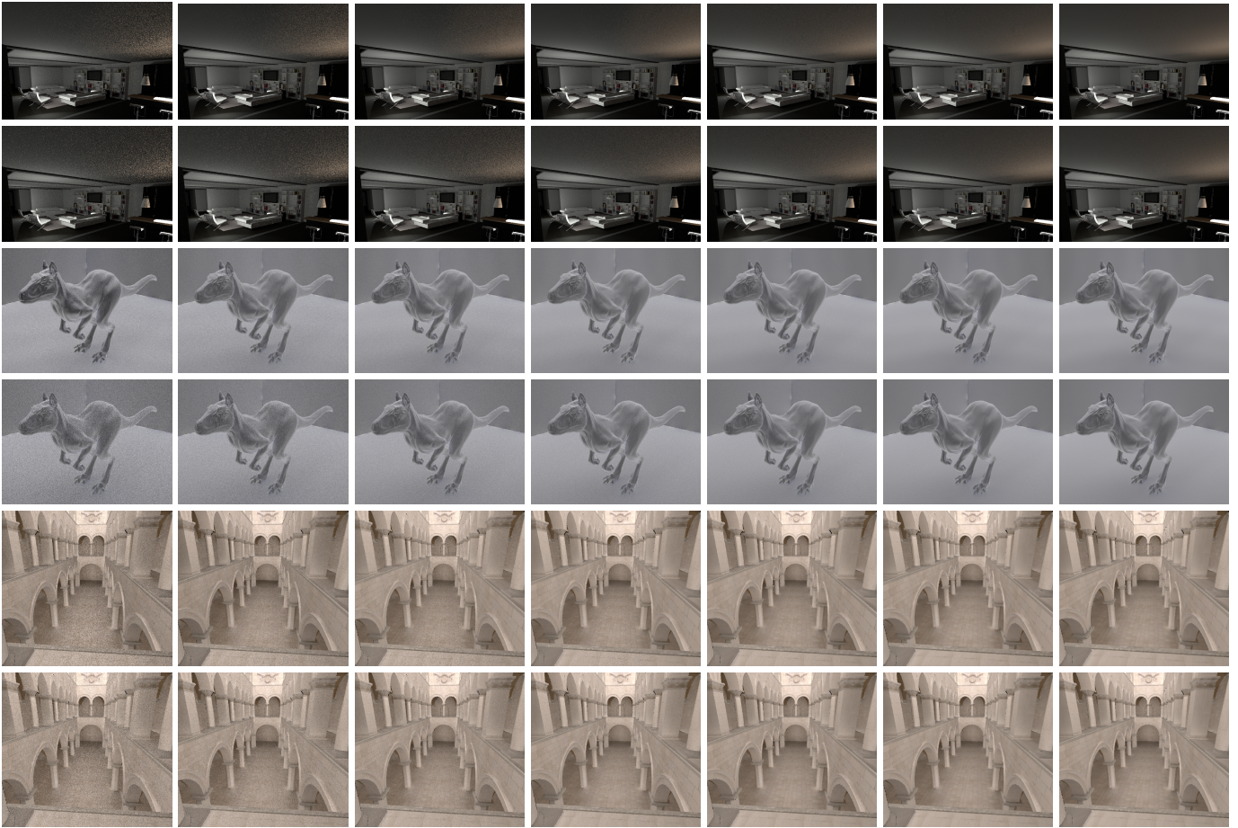
Figure 2: Experimental results for final gathering using our technique (top row for each scene) and classical final gathering (bottom row for each scene). The columns correspond to 16, 32, 64, 128, 256, 512, and 1024 samples in the hemisphere, respectively. See Fig. 1 for the corresponding error rates.
